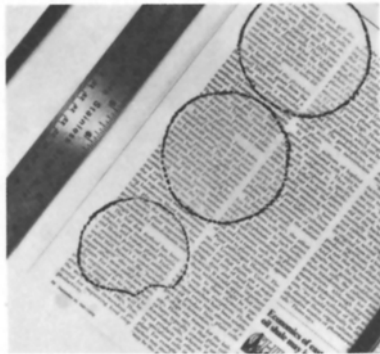
Fig. 1. Ceramer samples made with 48 wt% TEOS and 52 wt% PDMS(MW=1700)
